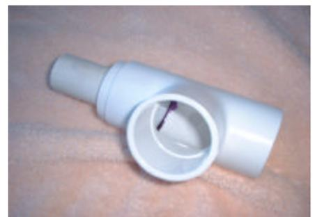
A short piece of 1 inch pipe was used for this particular install and it is glued in place. The reducer is glued into the T connector too. Note the black ring inside the adapter. That's the glue used to hold the baffle in place. On the next page is what it looks like actually installed on the vent pipe.
