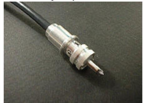
center conductor to the pin allowing some solder to wick back flowing into the pin interior a bit. Don't overdo it though.
