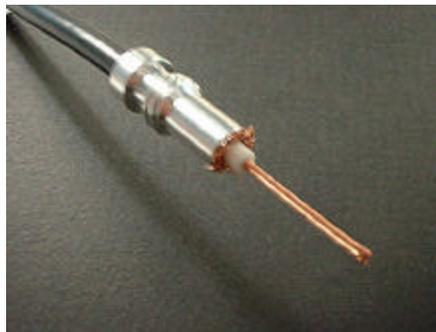
**Sixth**, carefully solder the braid to the end rim of the reducer all the way around the circumference. Try not to melt the center insulation any. It will take practice to develop this skill. Examine your work in particular noting the condition of the center insulation.
