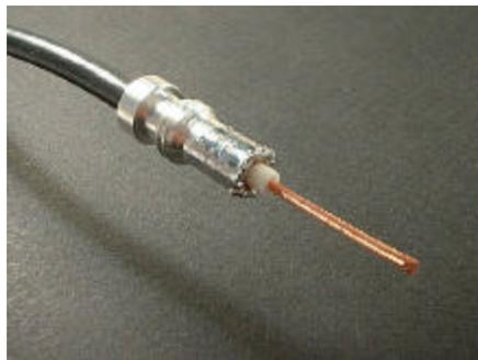
**Seventh**, examine the center insulation and, if needed, remove enough to leave 3/16 inch protruding.
