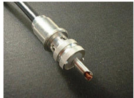
finger tight you can firm up the connection between the reducer and the shell of the PL259 using a couple sets of pliers. One on the reducer end and another on the PL259 serrated rings. Try not to mar the parts. This does not need to be gorilla tight.
