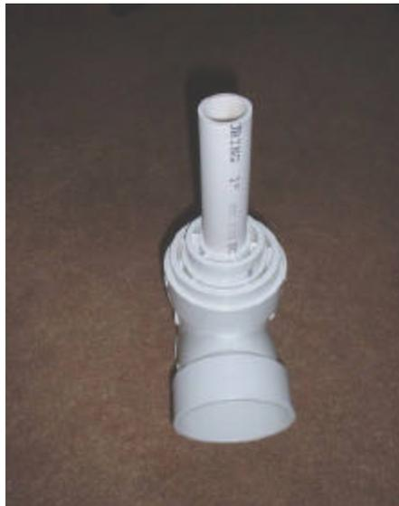
The next column shows the shroud in place. Of course, if you don't like creamy yellow you can select any color you desire or paint the thing any way you like. I would point out though that you should **not** paint the antenna itself. Doing so will change the operating frequency. The dimensions used here were arrived at specifically using 1 inch schedule 40 PVC pipe. Any substitutions or finish on the radome will change frequency. Design adjustments would be needed if a finish was to be
