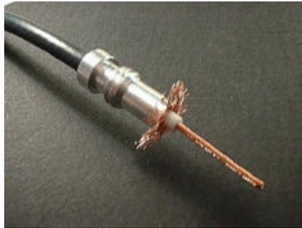
wife's sewing scissors) trim the shield wires so that they do not extend beyond the outer circumference of the reducer end. A very slight overlap is OK at this point but you'll just wind up trimming it off later so keep a tight tolerance.
