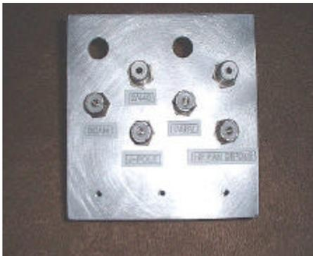
tify which antenna is connected outside. During thunderstorms I always disconnect all radio equipment from the antennas. Corresponding labeling on the cables from my radio switch panel make it easy to match up and reconnect everything in my radio area quickly.
