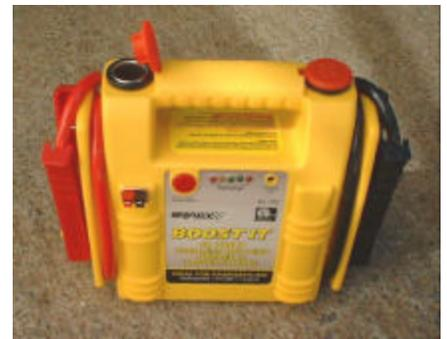
packs commonly seen at Wal-Mart or at the auto stores. They don't have much capacity but at a reduced transmit power setting on your transceiver it may do the trick for a while. I modified one I have by installing a set of Anderson Power Pole connectors on the side and wiring them to the sealed wet cell inside. This was done simply by using a little heavy wire, 2 ring con-
