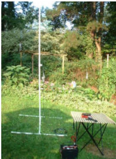
Here's a complete simple station set up in my yard ready to go. On the table is a 2 meter FM radio. On the ground is a car battery for power and the white object is a 2 Meter antenna I made and the PVC pipe antenna stand. Cables to connect it all together and a table for convenience and you're in business. Cost, sans the fold up table, is around \$ 270. A closer look reveals the car battery
